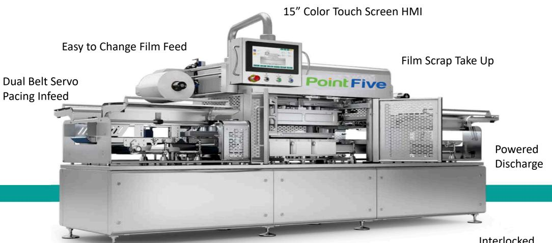
Heavy Duty Welded Stainless Steel Washdown Construction Reciprocating High Speed Tray Feed Mechanism
